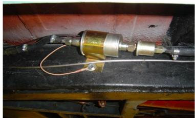
protect the wire from mishaps that may render it unusable. You will butt connect the wire to the remaining wire coming from the fuel pump.
