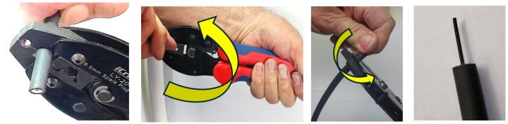
Keeping Wire straight, rotate the tool 360 degrees, 5-10 times to fully strip. You can also twist the other end a few times and it should come off with no nicks on the conductor
