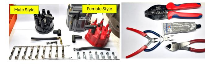
Older style distributor caps are often the Male style Termination and the Female Terminations are for HEI and MSD style distributor caps . You will need a Spark Plug Wire Crimping and Stripping Tool, Wire Cutters (large and small), as well as small pliers and Dielectric Grease
