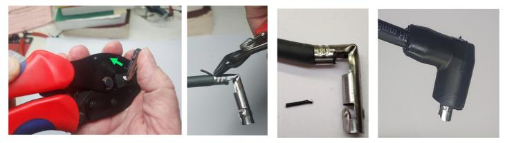
Reload the finished crimp into the tool, compress the handles and use your thumb to push the terminal end until it is 90 degrees at the fold. Trim the excess conductor from the back of the terminaland then using dielectric grease on the spark plug wire, pull the wire through the boot until it is firmly seated. Apply dielectric grease to each spark plug insulator, as you go, as this will make removing the spark plug wires easier in the future.
