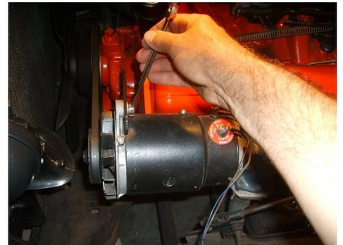
Remove adjusting brace hardware and remove belt. Remove lower mounting hardware and remove generator. Check bracket size in next step.
