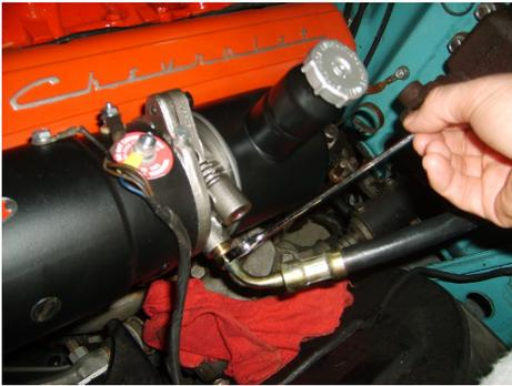
**9029** drain the pump down at the linkage, disconnect the hoses from the pump, plug ports. Remove the pump from the generator. **9029V** remove the tach drive unit.
