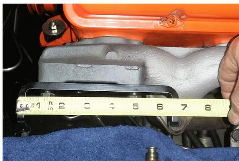
Verify the existing bracket length, measured from outside to outside of the mounting ears, use this chart to determine the correct length you need:
