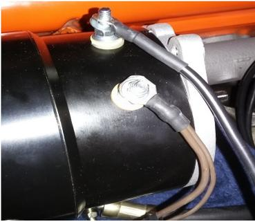
Install small end of new black charge wire to the terminal tagged "B+". Route charge wire to starter solenoid. **9029V** For installation with ammeter see special instructions.
