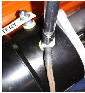
**9029, 9005**, for correct Dash Lamp operation, attach your existing double brown wire to the unlabeled alternator terminal (see pic). Insulate ends of remaining generator wires and tuck them into existing harness. **9029V** this terminal can be left bare or a dummy wire can be installed for appearances.
