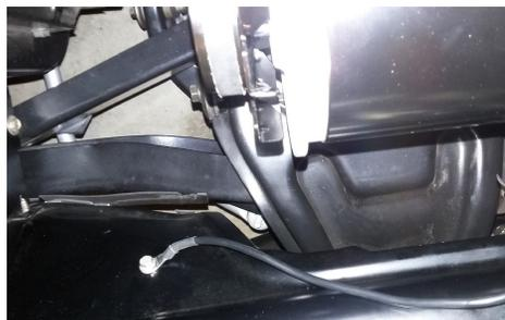
Install other end of ground wire to engine, frame, or front sheet metal. Be sure all OEM ground straps are installed on vehicle.
