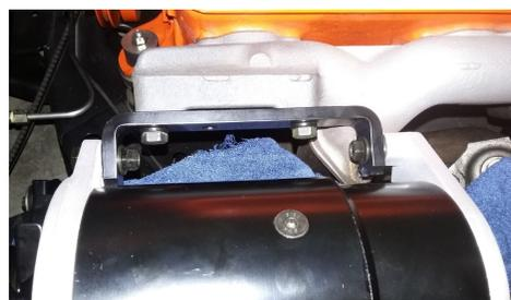
Install new alternator onto bracket using hardware provided. Install washers under the bolt heads and under the nuts.
