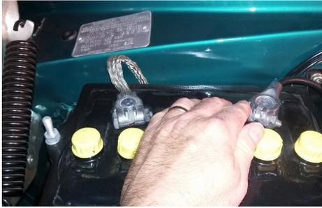
Make sure positive battery cable is connected, then connect negative battery cable, **SEE CAUTION NOTE ABOVE**. Start engine. GEN dash lamp should turn off after starting. Alternator does not need to be polarized.
