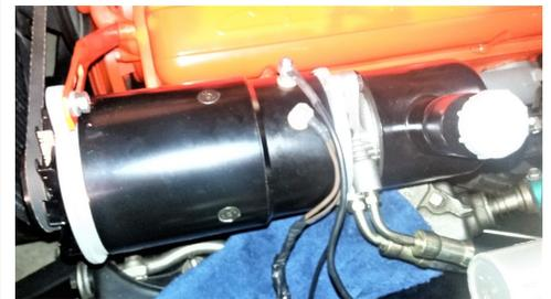
**9029** install all hoses at pump and at valve. Use line wrenches to tighten connections. **FILL PUMP WITH FLUID! USE**
