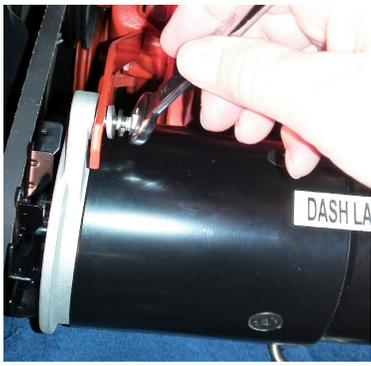
Install belt and adjusting brace with hardware provided. Tighten brace, tension belt as per shop manual.
