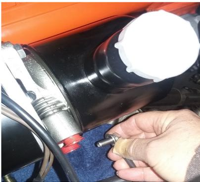
**9029** install pump using new hardware provided. With lower bolt, install one end of short ground wire.
