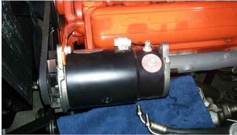
**On all generators**, remove all the wires from the generator. Do not cut wires. Lay wires aside.
