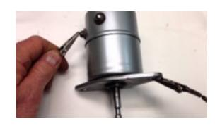
while. But a 12 volt solenoid will not operate on 6 volts. Be careful when buying used solenoids in the open market, you may not be buying a 12 volt solenoid and you may get a 6 volt solenoid and find that it fails after a short time on 12 volts.
