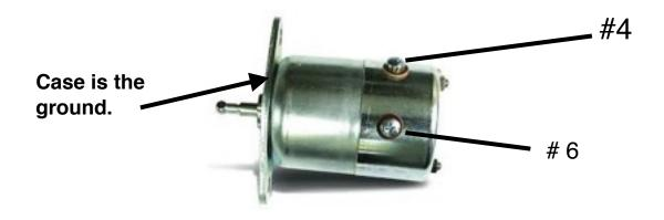
There were two solenoid manufactures besides Borg Warner which were Autolite and Delco. Both of these will interchange as long as the shaft length matches and the operating voltage is correct with your vehicle.
